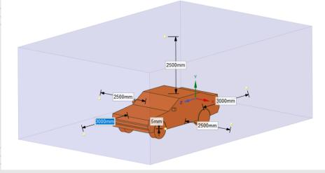
When deciding on making the enclosure, key design considerations were based on the boundary layers. For the front and back of the enclosure we made the lengths 3000mm as they are the inlet and outlet boundary layers, respectively.
