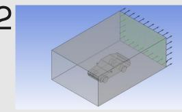
Figure 7: Isometric view of the outlet boundary layer Boundary layer name: Outlet Type of flow: Subsonic Average Static pressure: 0 Pa
