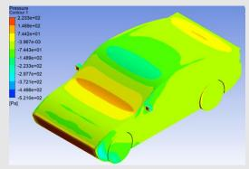
Figure 26: Isometric view pressure contour
