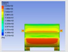
Figure 30: Front view pressure contour
