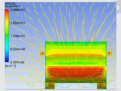
Figure 31: Front view velocity streamlines
