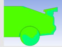
Figure 35: Side view pressure contour
