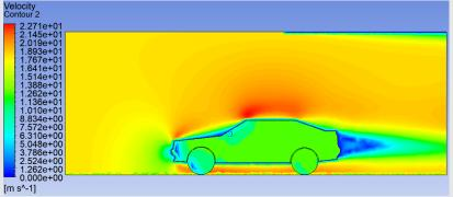
Figure 46: Side view velocity contour
