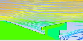
Figure 38: Closeup view of velocity streamlines across spoiler addition
