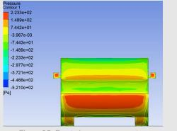
Figure 25: Front view pressure contour
