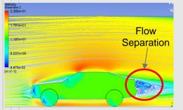
Figure 14: Pressure Contour and Streamlines (Side)
