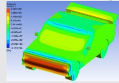
Figure 39: Isometric view pressure contour
